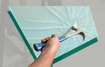
Toughened glass is manufactured by heating and rapidly cooling annealed panes, a process known as thermal tempering.
