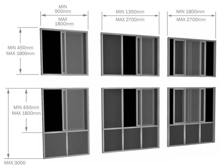
NO INDIVIDUAL PANEL MAY EXCEED 2.4 sq. m IN AREA, OR 2400mm IN ANY DIMENSION OUTER FRAME CANNOT EXCEED 3000mm IN EITHER HEIGHT OR WIDTH
