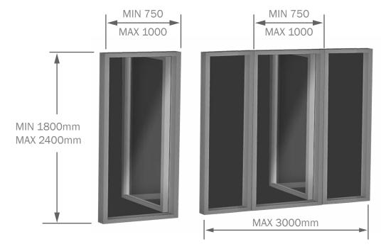
OPEN-IN, 1 PANEL CONFIGURATION ONLY (NO FRENCH DOORS). NO INDIVIDUAL PANEL MAY EXCEED 2.4 sq. m IN AREA, OR 2400mm IN ANY DIMENSION
