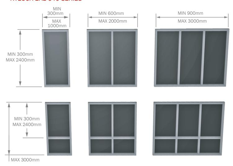
NO INDIVIDUAL PANEL MAY EXCEED 2.4 sq. m IN AREA, OR 2400mm IN ANY DIMENSION HEIGHT & WIDTH CAN TYPICALLY BE REVERSED
