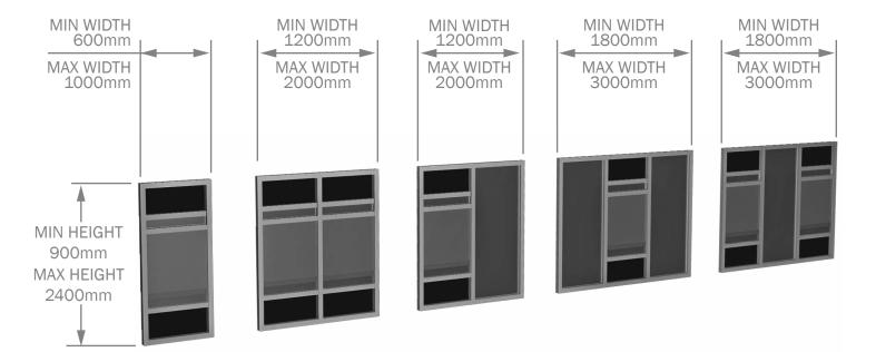
NO INDIVIDUAL PANEL MAY EXCEED 2.4 sq. m IN AREA, OR 2400mm IN ANY DIMENSION PRODUCT WIDTH CAN NEVER EXCEED HEIGHT OUTER FRAME CANNOT EXCEED 3000mm IN EITHER HEIGHT OR WIDTH
