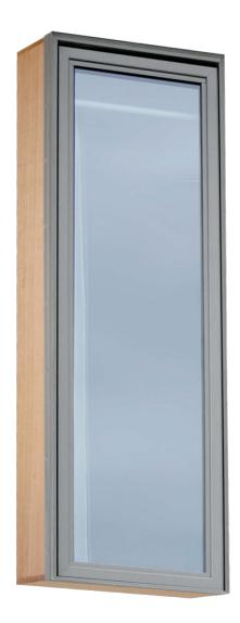
To ensure a tight seal when closed, two separate mechanical latches clamp the sash tightly against the outer frame. The dual seals surrounding the perimeter of the sash are then able to effectively exclude wind & water.
